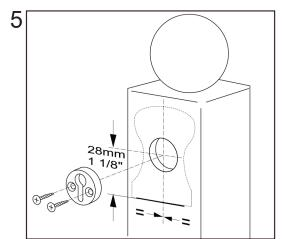
To mark the centre of the keyhole disc measure 1 %" (28 mm) upwards from the bottom of the rail position. Using a 1" (25 mm) bit bore hole into post \$32" (7 mm) deep so the keyhole disc is flush or slightly under. Secure disc with screws, bore pilot holes first.
