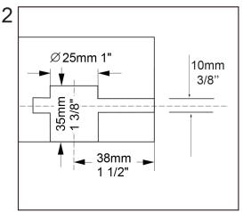
Mark and bore 1" (25mm) hole first then bore 3/8" (10mm) hole.
