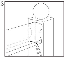
Mark fully final position of the handrail onto post observing the centre line.
