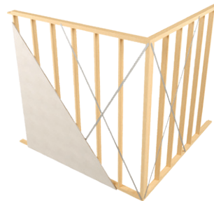
Typical RWB/WB installation
