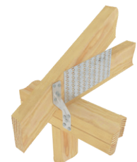
Typical RT7A truss/rafter to double plate installation
