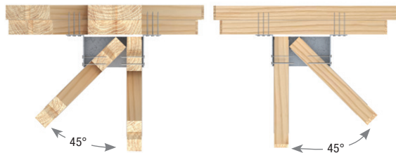
Typical HJC/HTHJ installation top view
