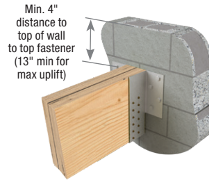
Typical HGUM installation
