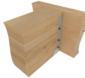
Typical HDQIF inverted flange installation
