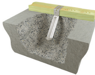
Alternate FA3 installation (concrete slab only)
