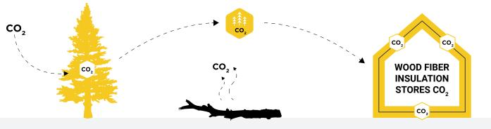
Atmospheric carbon dioxide is taken up by trees and, through photosynthesis, is stored as carbon in biomass At the end of a tree's life, when left to decay, this stored carbon will return to the atmosphere slowly Using residual wood chips and low-grade softwood trees as the source material for wood fiber insulation locks in carbon for the lifetime of the building
