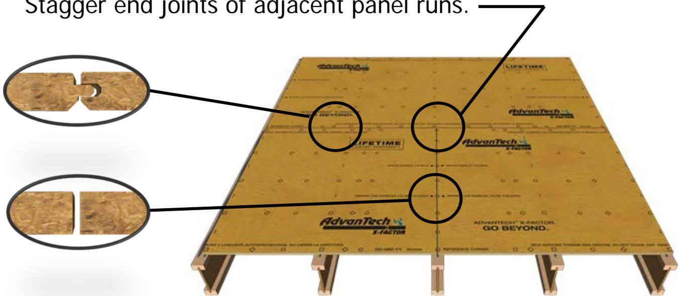
PRO TIP: use 10d nails to space the AdvanTech X-Factor subfloor panels 1/8-inch.
