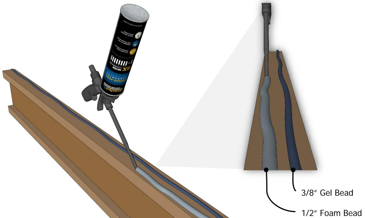
Where two subflooring panels come together on the same joist, apply two lines of adhesive to ensure both panels will have adhesive.
