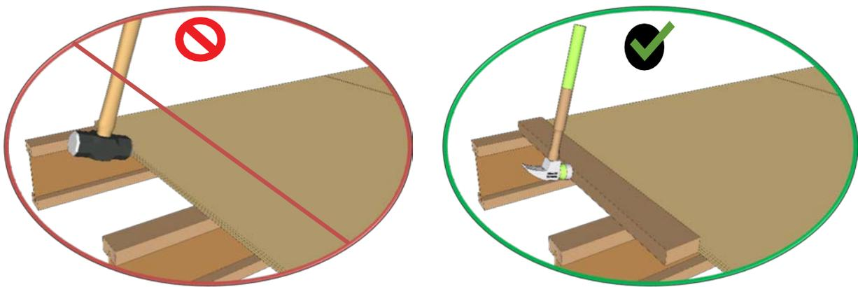
**PRO TIP:** Install the first row of AdvanTech X-Factor subflooring with the tongue profile oriented towards the exterior. This allows for the wooden block to be placed on the groove when tapping the panel into place. This prevents crushing of the tongue.
