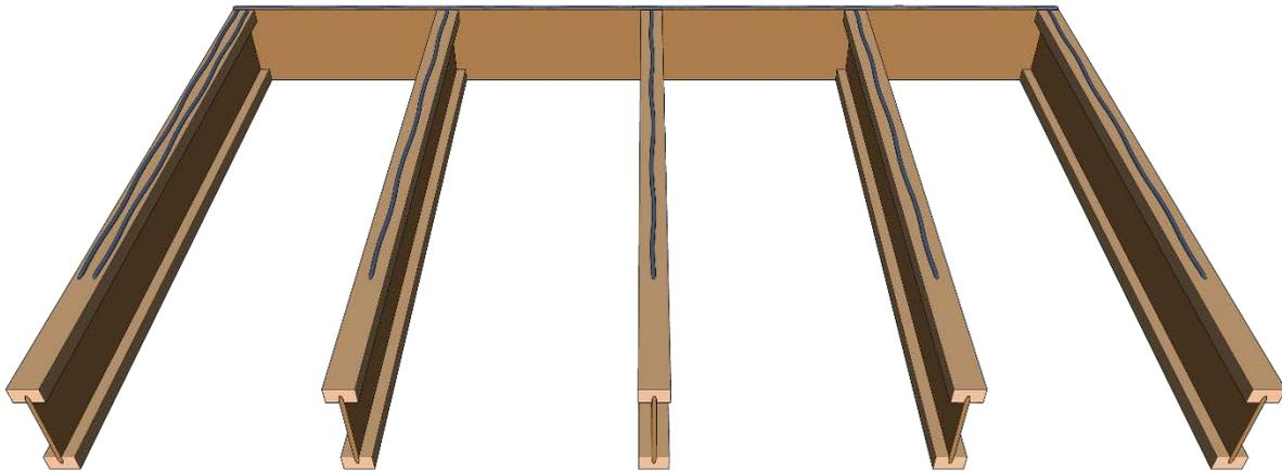
Immediately after applying the adhesive, lower the panel into place, making sure the panel is square on the joists. The top side of the panel should be facing up to allow for the certification stamp to be easily viewed from the bottom by local building officials. Panels should span two or more spans (three or more floor joists) with the long dimension perpendicular to the floor framing.
