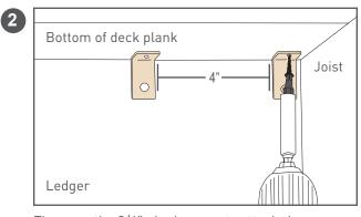
Then use the 3/4" plank screw to attach the L-Bracket to the underside of the plank.
