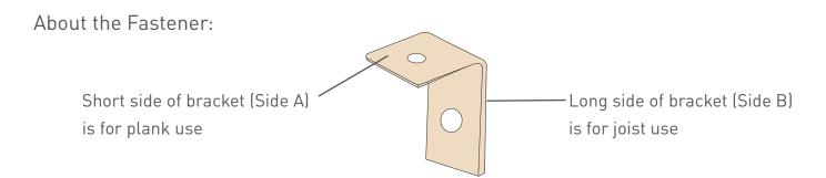
Clip Spacing: For either installation option, locate and install one L-Bracket at the start and end of the plank in the corner where the joist meets the rim joist. Then install two clips in every joist bay spaced where x = J/2 and y = J/4 where (J) is the center to center spacing of the joist.
