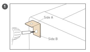
Use the 1-1/2" joist screw provided to install the L-Bracket into the outside of the rim joist.
