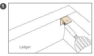
Use the 1-1/2" joist screw provided to install the L-Bracket into the inside of the rim joist.
