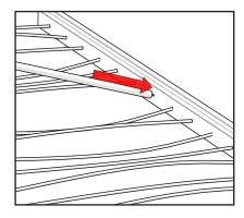
View the chart to determine the rods' positions, cut and remove unnecessary cables, then insert rods into empty holes.
