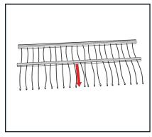
Unwrap cables and lay section flat (on a non-abrasive surface). Then spread Rails tightly to each end.
