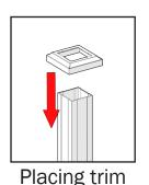
Space Posts according to \*application and Top Rail length. Place leveling plate (highlighted) between Post and mounting surface.
