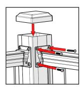
Ensure Top Rail is correct height from deck surface (check both sides).
