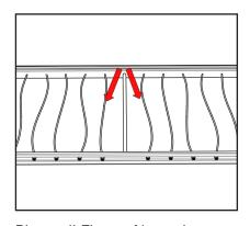
Place all Flange Nuts, then finger tighten the Nuts of only the cables adjacent to each Support Rod.
